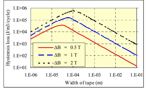
Figure 4. Hysteresis loss as a function of tape width for various magnetic fields in YBCO tape.
