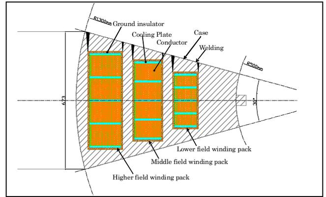
Figure 7. Cross-section of the winding at the mid-plane in the inner leg.
