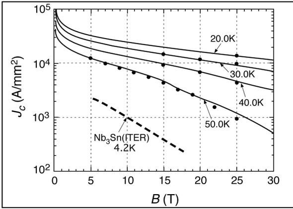
Figure 2.  $J_c$  vs.  $B$  performance for YBCO tape compared to the  $Nb_3Sn$  strand applied to ITER.
