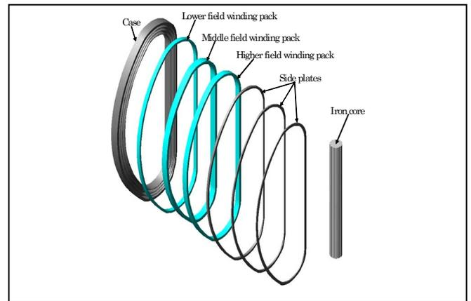
Figure 8. Expanded view of a TF coil
