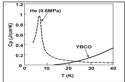
Figure 5. Specific heat as a function of temperature in YBCO material in comparison of supercritical helium.
