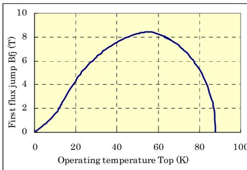
Figure 3.  $B_{fj}$  as a function of the operating temperature ( $T_o$ ) in YBCO tape.
