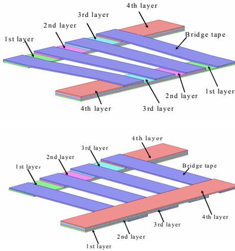
Figure 9. Joint configuration. (a) : pancake-to-pancake joint (upper) and (b) : double pancake-to-double pancake joint (lower).
