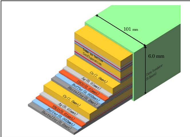
Figure 6. A 20 T 40 kA 33 K YBCO conductor
